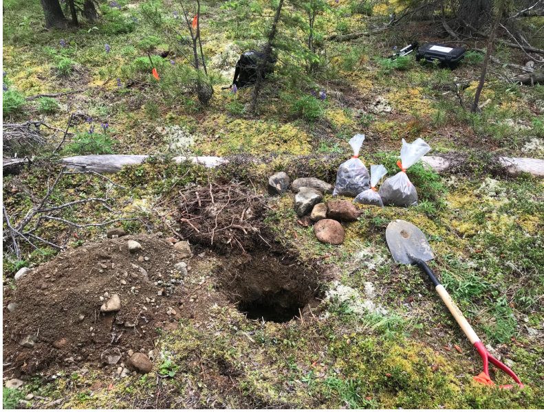
Figure 7 – Photograph of sampling site 20MK-010 on June 18, 2020. Glaciofluvial gravel overlying Mandanna member of the Aksala Formation (sandstone and conglomerate). Three bags of sediment, from left to right, for clast lithology/geochemical analysis, matrix geochemistry, and grain size distribution. The spectrometer case is visible in top right and a probe flagged with orange tape can be seen in the top left.
