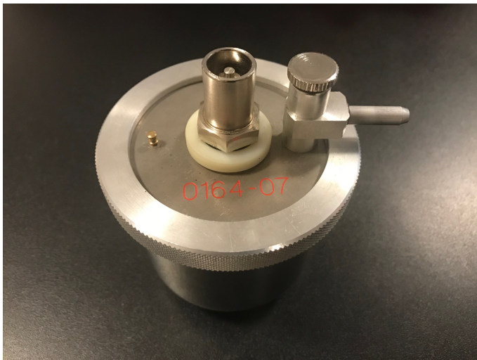
Figure 9 – IK-250 ionization chamber for radon concentration measurement, 250 ml capacity. Serial number is red, electrodes are brass pin at left and silver pin in central cylinder. Valve at right (knob above protruding tube).
