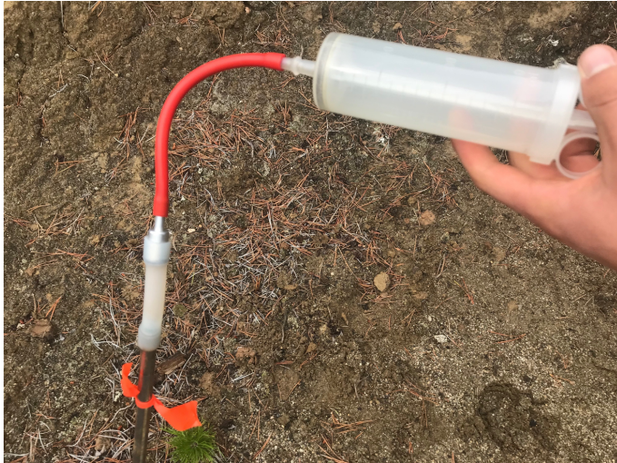
Figure 8 – Soil gas extraction using 150 ml syringe. Red rubber tube connects directly to valve on ionization chamber. Probe flagged with orange tape.
