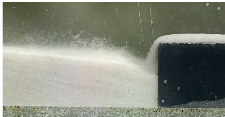
Figure C.3: Image taken with the Olympus camera showing the scour pit formed at the upstream end of the well during a S1 trial (no seeding in this case). Flow is from right to left. Note the suspended sediment moving in the water column above the bedload layer. For scale, the thickness of the PVC plate is 2.6 cm.
