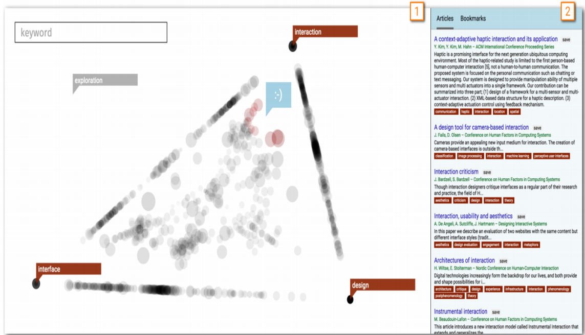
Figure 2.2: Visual Re-Ranking for Multi-Aspect Information Retrieval: The interactive relevance map is rendered based on three topics selected shown in the red label, and one topic disabled is greyed out. The user can select the exploration cursor (in blue) to select the region for re-ranking the documents. Documents rendered as red points are the top documents retrieved in rank list [18].
