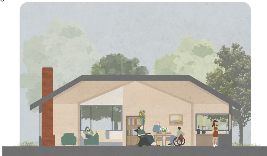
Section cut of large cabin through living space, dining space and kitchen
