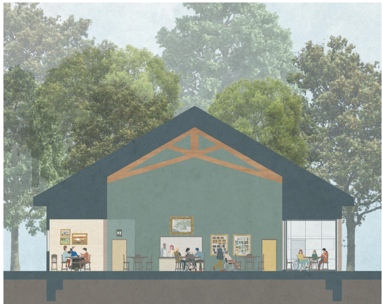
Section of dining space in the lodge with dropped ceilings to make smaller, more comfortable spaces
