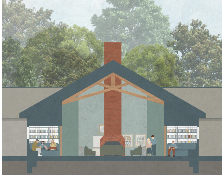
Section of activities space in the lodge with dropped ceilings to make smaller, more comfortable spaces
