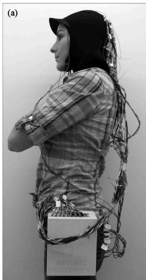
Figure 6-4. Example of a mobile fNIRS system utilizing APDs. 18
