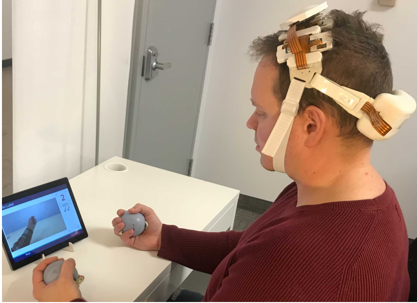
Figure 5-1. Illustration of the experimental set up for the present study. Participants wore the fNIRS prototype headband while a movement video played a fist squeezing task on a tablet. Participants were asked to follow along with the movements in the video as best they could.
