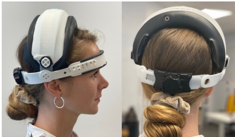
Figure 6-5. Axem Home headband prototype as of January 2021. This prototype includes a one-time adjustable forehead strap that is sized depending on the head size of the wearer (i.e., this strap would only need to be sized by the wearer upon first use), as well as an adjustable band back that allows for a snug fit to be achieved each time they don the device.
