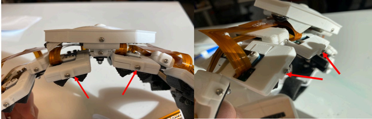
Figure 2-9. Illustration of the spring attachment design, allowing the individual LED pods (example of these pods are pointed to with red arrow in figure) to articulate in the sagittal plane, independent from the central headband.
