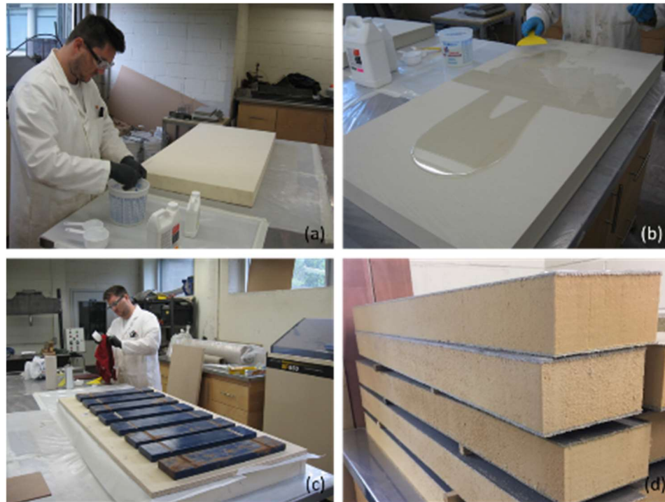
Figure 3-1. Specimen fabrication: (a) mixing epoxy and section of cleaned foam; (b) application of epoxy; (c) specimen curing with weighted board; and (d) finished specimens
