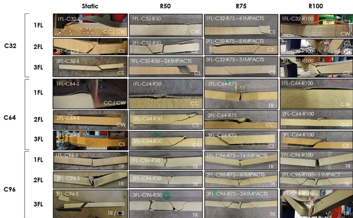
Figure 4-4. Failure modes of all specimens [Note static specimens were tested as a part of another study by Betts et al (2018)]
