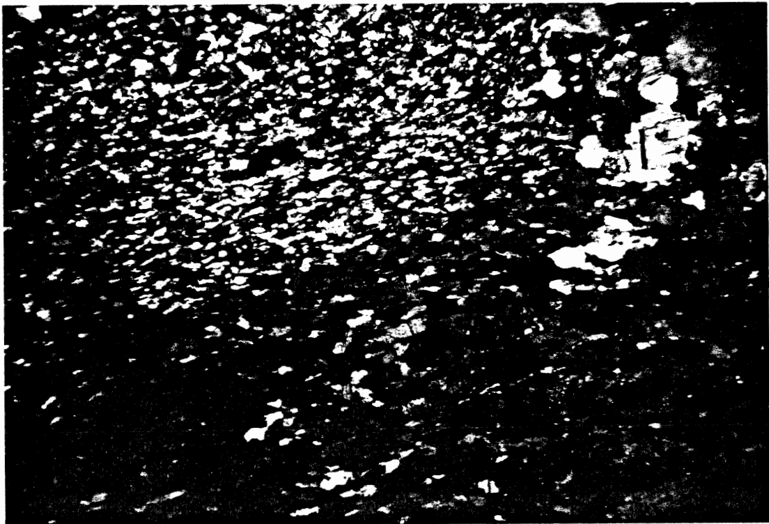
FIGURE 3.2 Calc-silicate showing mafic-rich and felsic-rich zones. Mafic-rich zones contain >90 percent hb and cpx, felsic-rich zones contain equal amounts of plag and hb. XN, scale 4*1.25
