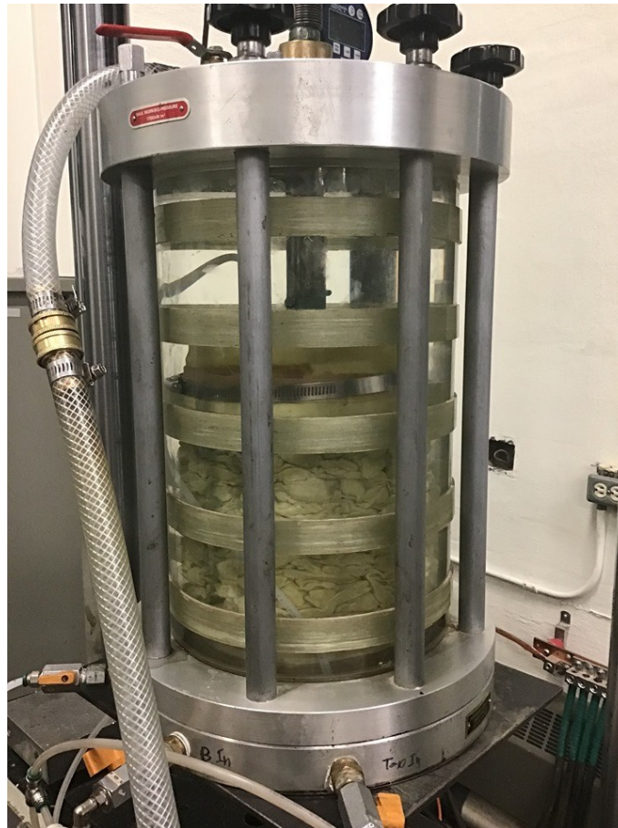
Figure 5.3 The sample deformation at 20% strain
