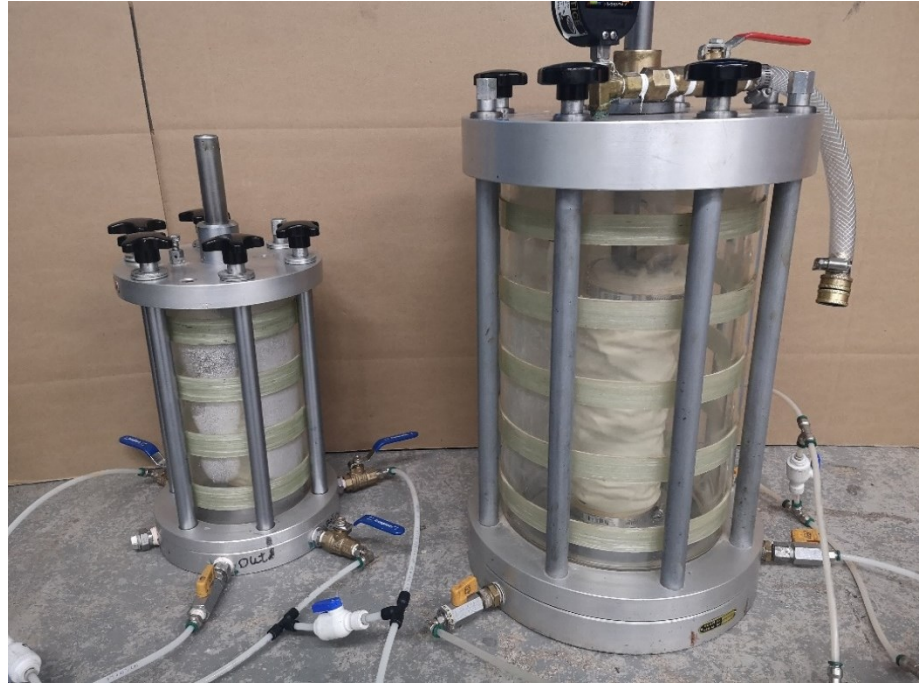
Figure 5.2 The Triaxial apparatus used in the study
