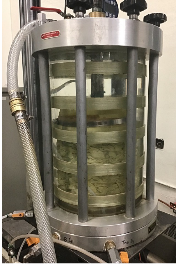
Figure 6.4 The sample deformation at 20% Strain
