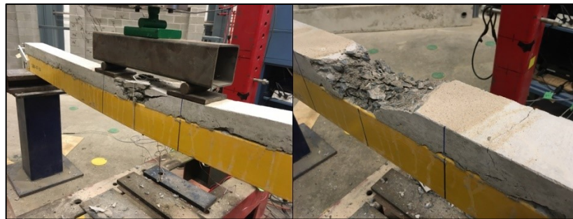
Figure 3-30 Pictures of SSA2-55-03 after concrete crushing failure due to four-point bending
