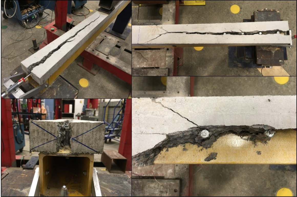
Figure 3-31 Pictures of SSB2-55-01 after concrete tensile failure due to four-point bending
