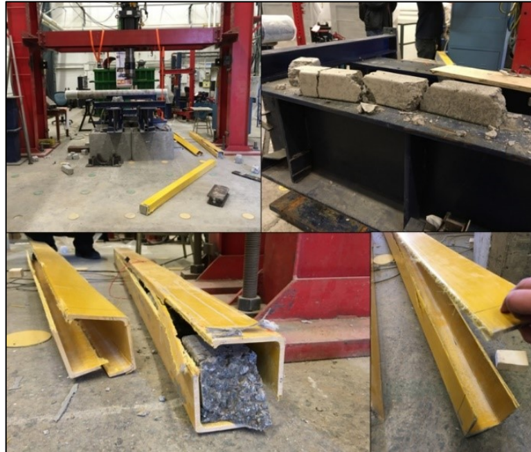
Figure 3-27 Pictures of the filled specimen FS2x3-01 after failure under four-point bending
