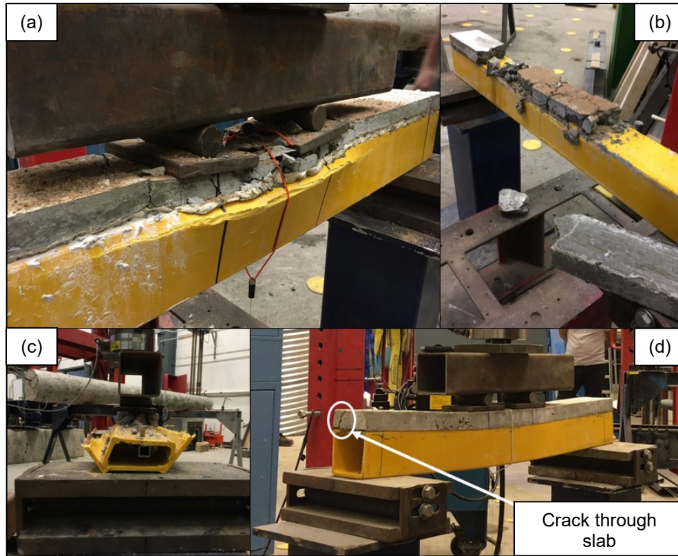
Figure 3-28 Pictures of 1 m long slab specimens after failure due to four-point bending: (a) SSA1-35-02, (b) SSC1-35-01, (c) SSB1-35-01 and (d) SSB1-35-02 (just before FRP failure)
