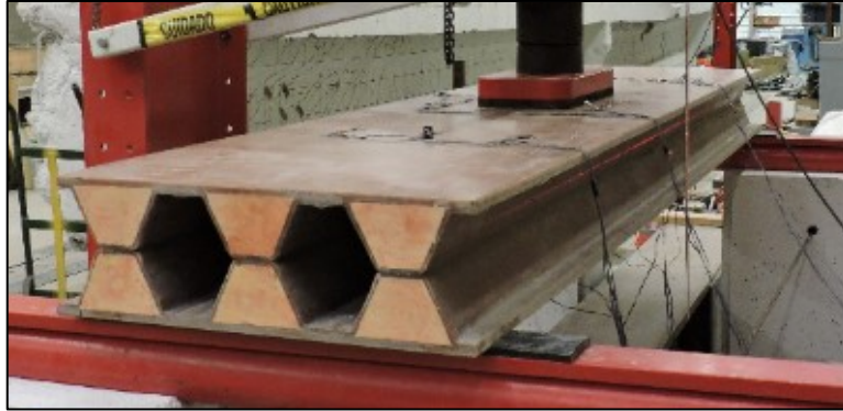
Figure 2-7 FRP deck profile with foam-filled sections (Volz et al. 2017)
