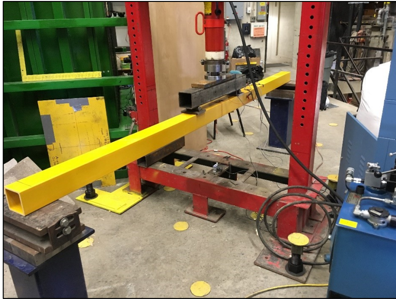
Figure 3-21 Picture of four-point bending test set-up for hollow specimen HS3-01
