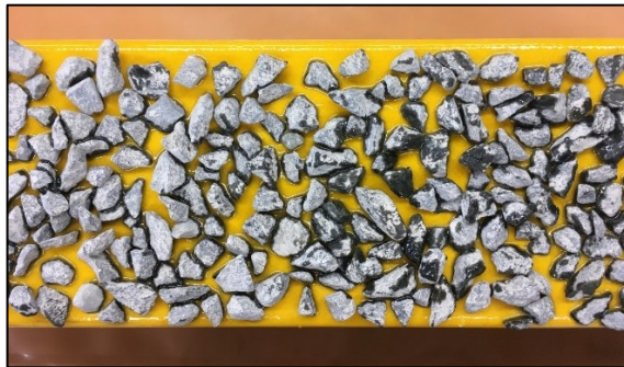
Figure 3-18 Aggregate set in epoxy on top face of FRP section
