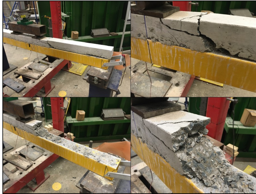
Figure 3-29 Pictures of SSA2-75-02 after concrete bond failure due to four-point bending
