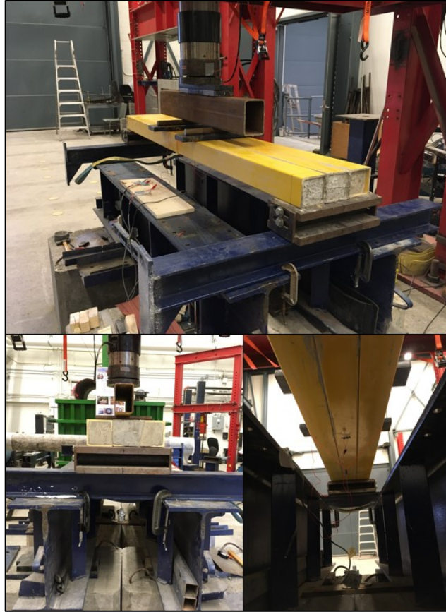
Figure 3-22 Pictures of four-point bending test set-up for the filled specimen FS2x3-01
