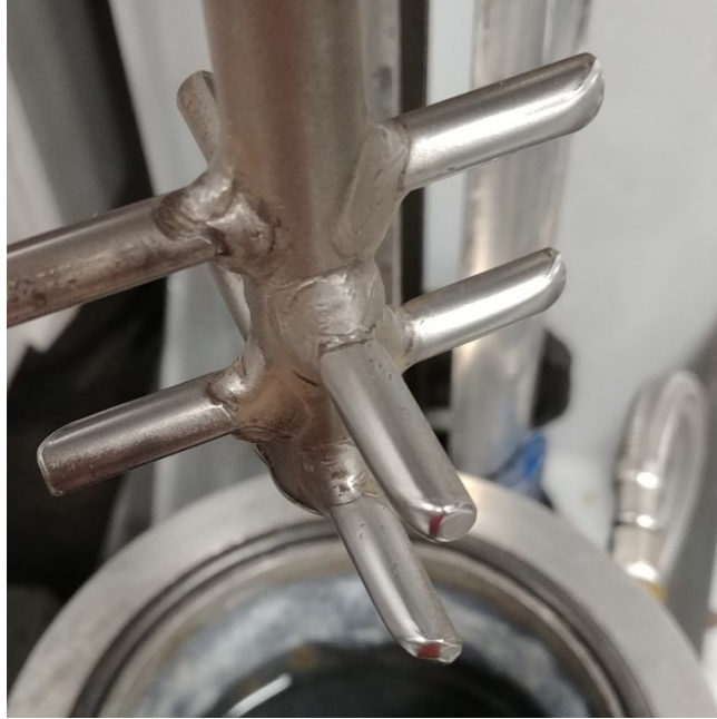
Figure 4-3 – Evidence of attritor arm wear causing unwanted Fe contamination in the \text{SiO}_x powders
