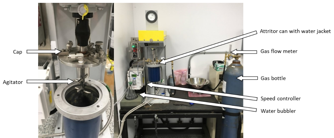
Figure 2-10 – Full attritor mill setup labeled and indicated as used on the Dalhousie Engineering campus
