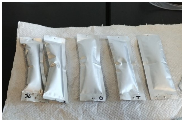
Figure 3-7 – Periodic \text{SiO}_x sampling and testing by the KOH method shows less \text{H}_2 is produced as more \text{SiO}_2 is formed while ball milling
