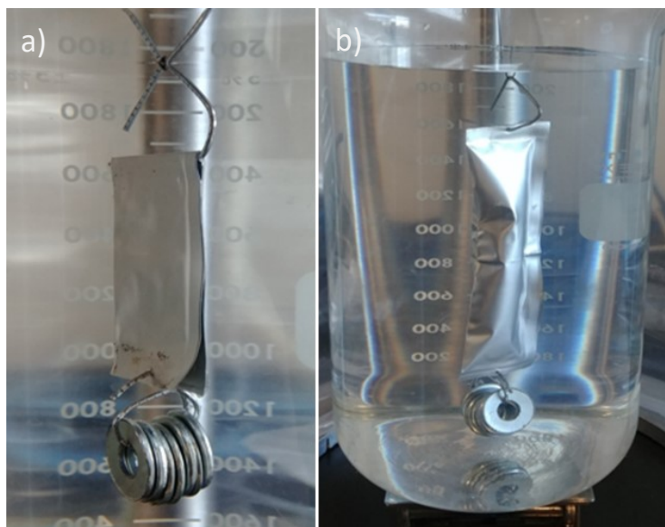
Figure 3-6 – a) Unreacted pouch bag with KOH and SiO x materials separated, b) Reacted pouch bag measuring hydrogen gas evolution
