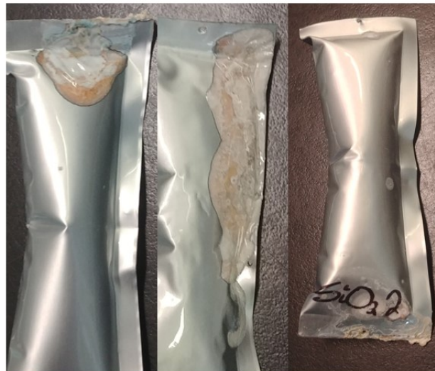
Figure 3-9 – KOH pouch bag deterioration due to reaction between pouch bag aluminum and KOH solution
