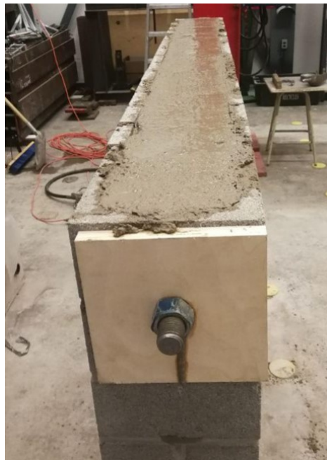
Figure 3.15 Threaded rod in the top beam
