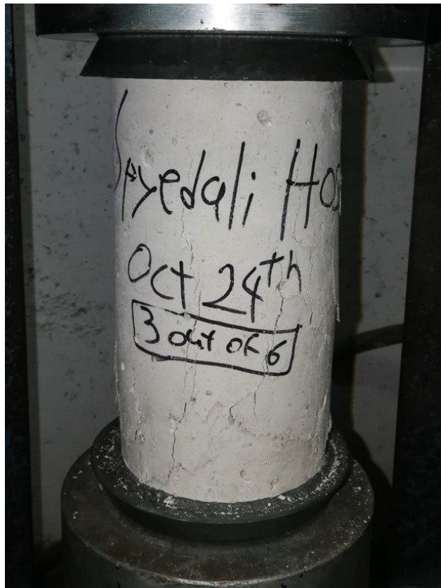
Figure B.6 Concrete cylinders failure pattern
