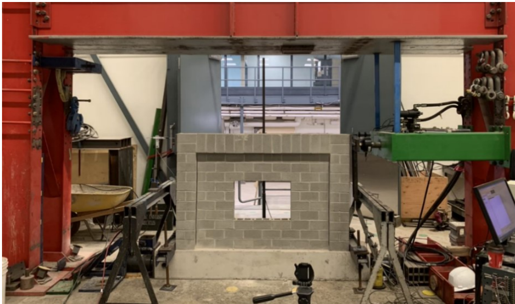
Figure 3.19 Cyclic loading setup
