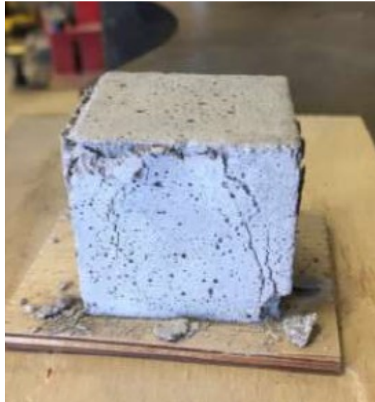
Figure B.2 Typical failure mode for mortar samples
