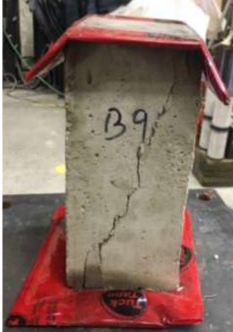
Figure B.3 Grout sample failure mode
