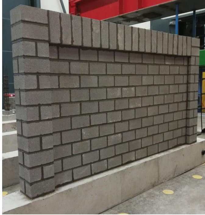
Figure 1.1 The proposed all-masonry infilled frame
