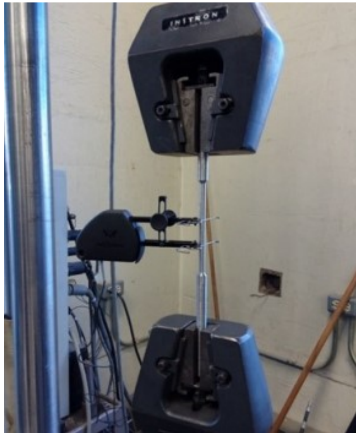
Figure A.9 Tension test set-up for steel coupons (Hu 2015)
