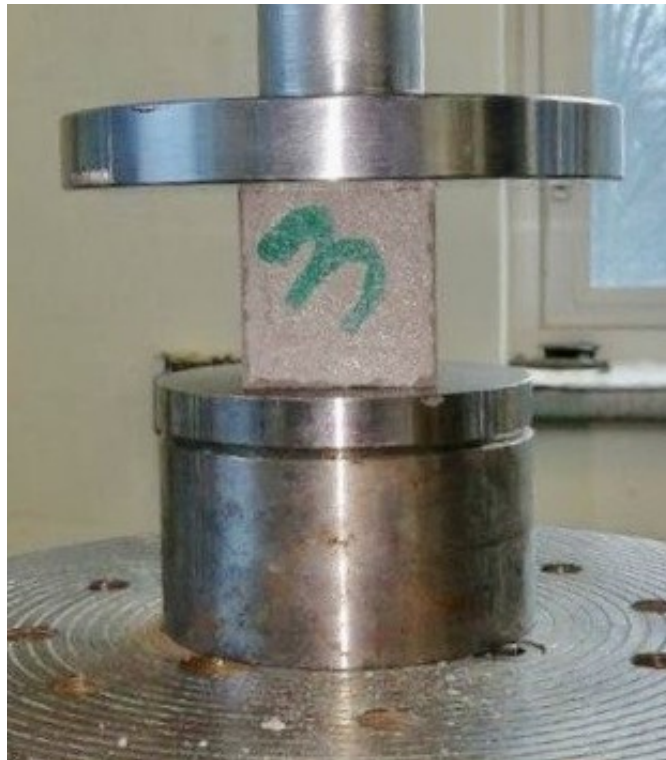
Figure A.2 Mortar samples under compression test
