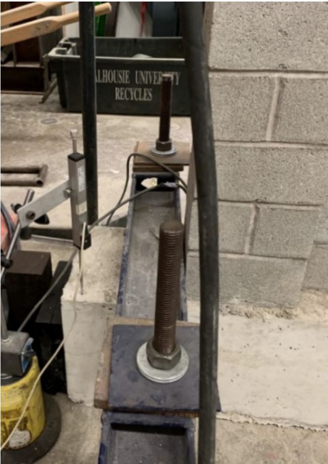
(a) Beam to floor clamping connection
