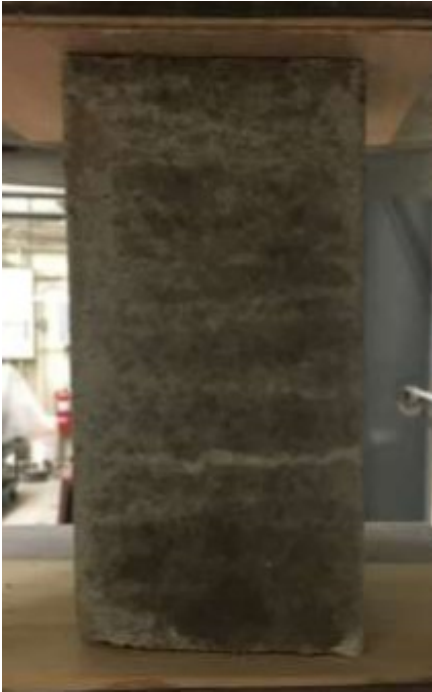
Figure A.4 Grout samples for compression test
