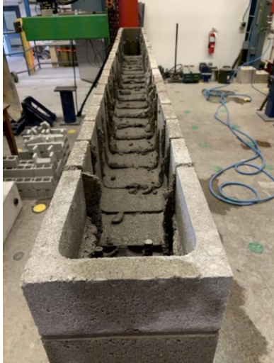
(a) U-shape blocks for top beam
