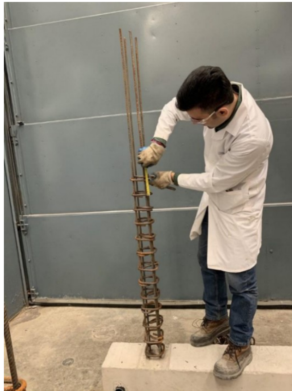
Figure 3.10 Tying stirrups on the column vertical rebars
