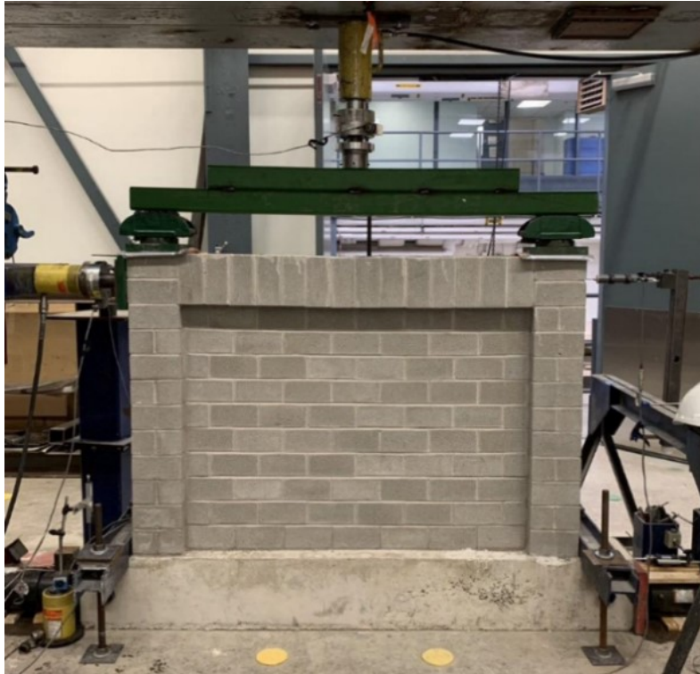
Figure 3.22 Combined vertical and lateral loading setup
