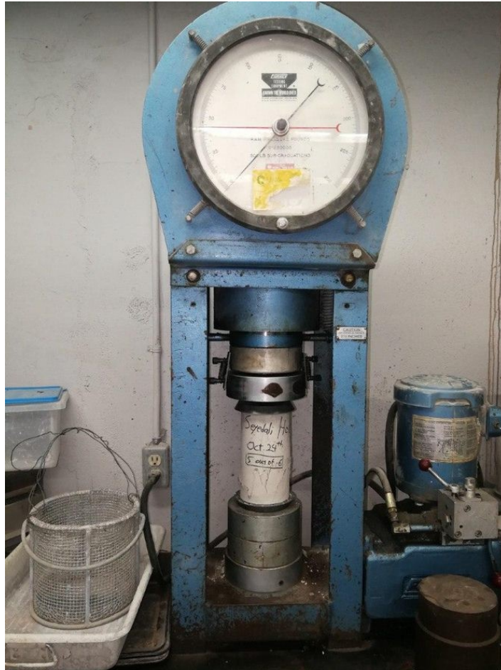
Figure A.7 Compression test setup for concrete cylinder
