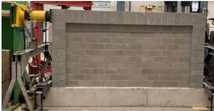
Figure 3.16 Lateral loading setup
