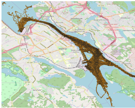
(a) Plotting 766,671 trajectory points generated by a vessel voyaging in Halifax waters.
