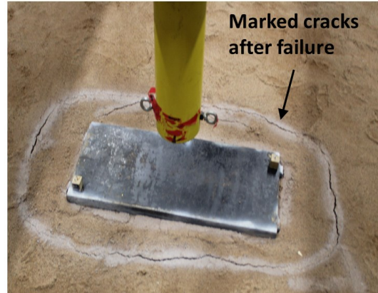
Figure 6-8 Failure mechanism for tests configurations 1 and 2
