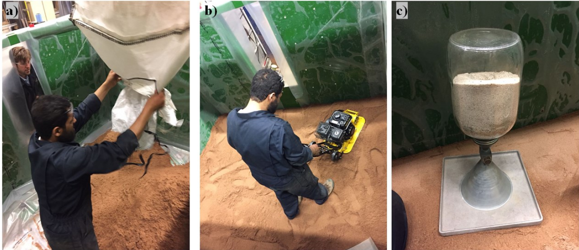
Figure 5-6 Backfill compaction procedures
