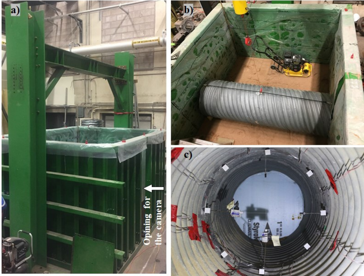
Figure 5-2 Test components: a) steel tank, b) corrugated culvert, and c) culvert instrumentations
