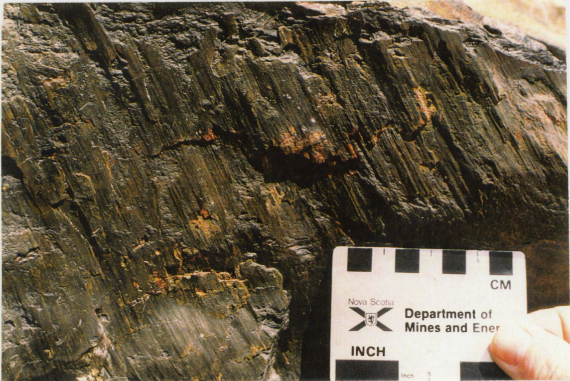
Figure 2.6 Slickenfibres on a bedding-concordant flexural-slip movement horizon showing the direction of flexural-slip movement (Photo courtesy of R. Horne, Nova Scotia Department of Natural Resources).
