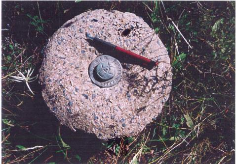
Figure 3.3 Photos showing a good gravity station with a control monument and its marker. Often the marker is not present or the control monument is damaged or missing.
