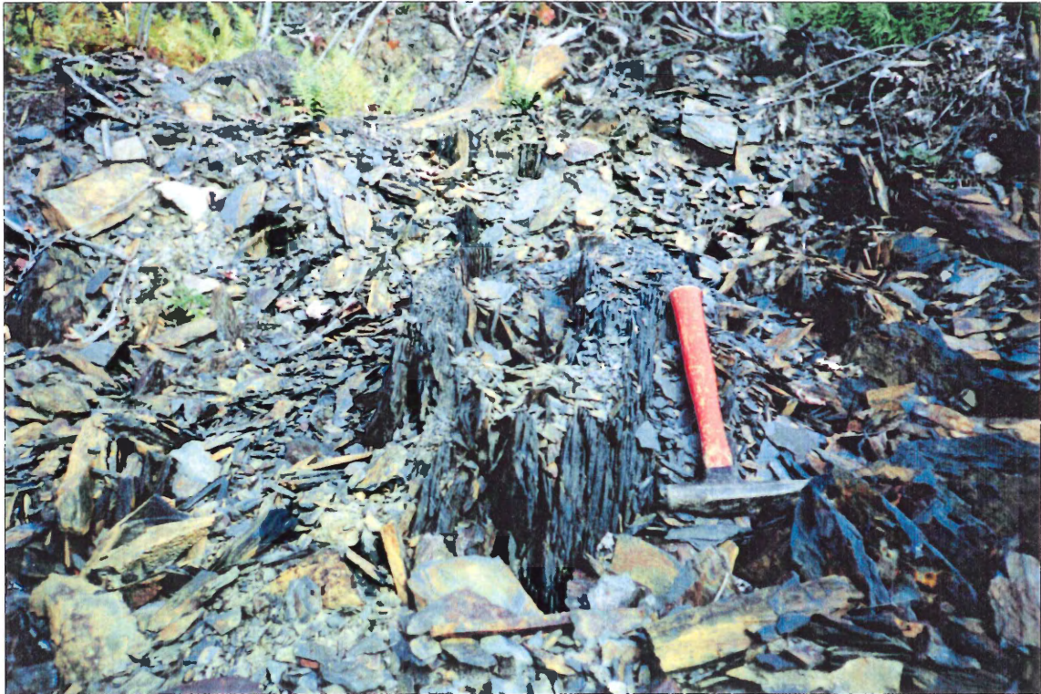
Figure 2.7: Typical well-cleaved, black slate of the Halifax Formation. Photo taken at Beaverbank Highway site at the location of sample CR-95-008.
