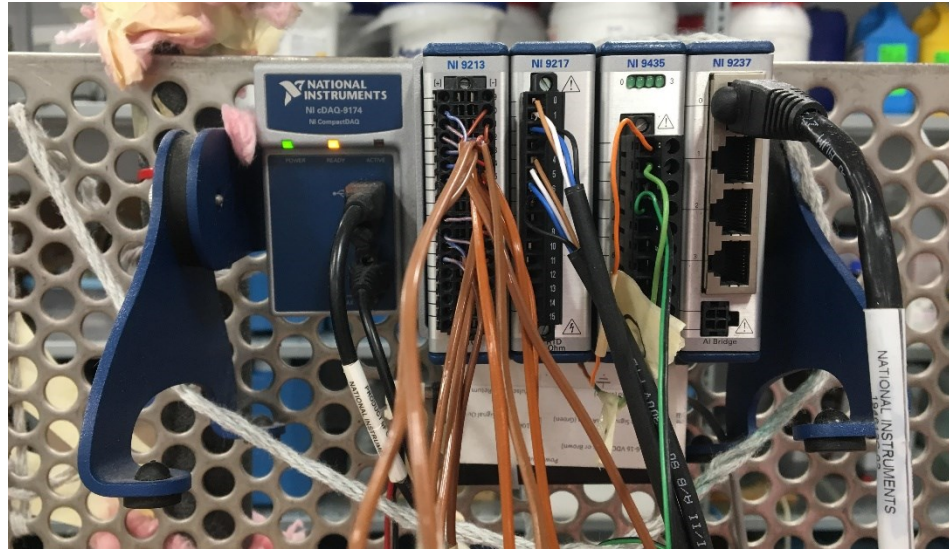
Figure 2.10: Picture of the NI-cDAQ 9174 chassis with the NI9213, NI9217, NI9435 and NI9237 modules mounted on it.
