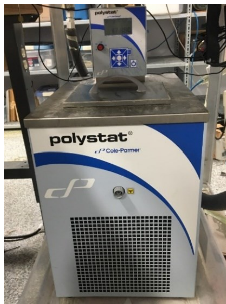
Figure 2.4: Picture of the Cole-Parmer Polystat RK-12122-56 heating and cooling circulating water bath.
