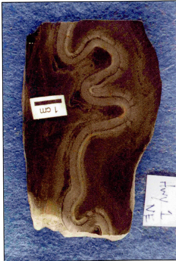
Figure 3.30. Slab photograph and sketch. Folds are symmetric to mildly asymmetric. Note that outer-arc extension is very well developed in the fold crests. Outer-arc extension indicates that the folds were formed when layers were stiff. The pattern of the outer-arc fractures indicates that these folds formed by tangential longitudinal strain during layer parallel shortening.
