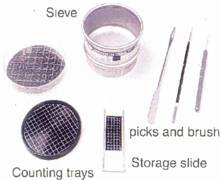
The above devices are used to ease the counting process. Sieves separate material of different sizes, counting trays allow the counter to keep track, picks and brushes are used to move the material around. (after Scott et al., 2001)
