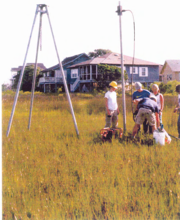
Figure 3.1. Vibracore set up. To the left is a tripod used for retrieving the core. On the right is the aluminum pipe, which will hold the core, once in the ground. -Photo taken from Dalhousie University southeastern United States Honors field trip, September 2000.
