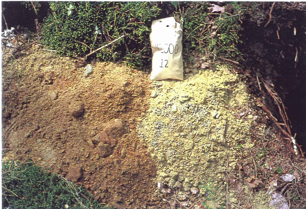
Figure 4.1 (Top Photo) Large plastic bags were used to collect 5 Kg till samples for clast identification and counts. The smaller kraft size sample bag was used to collect a ~ 500 g sample for geochemical analysis. (Lower Photo) Till samples used for this study come from the relatively unoxidized tan coloured till from the c-horizon on the right. The red brown till on the left overlies the unoxidized till and was not sampled.
