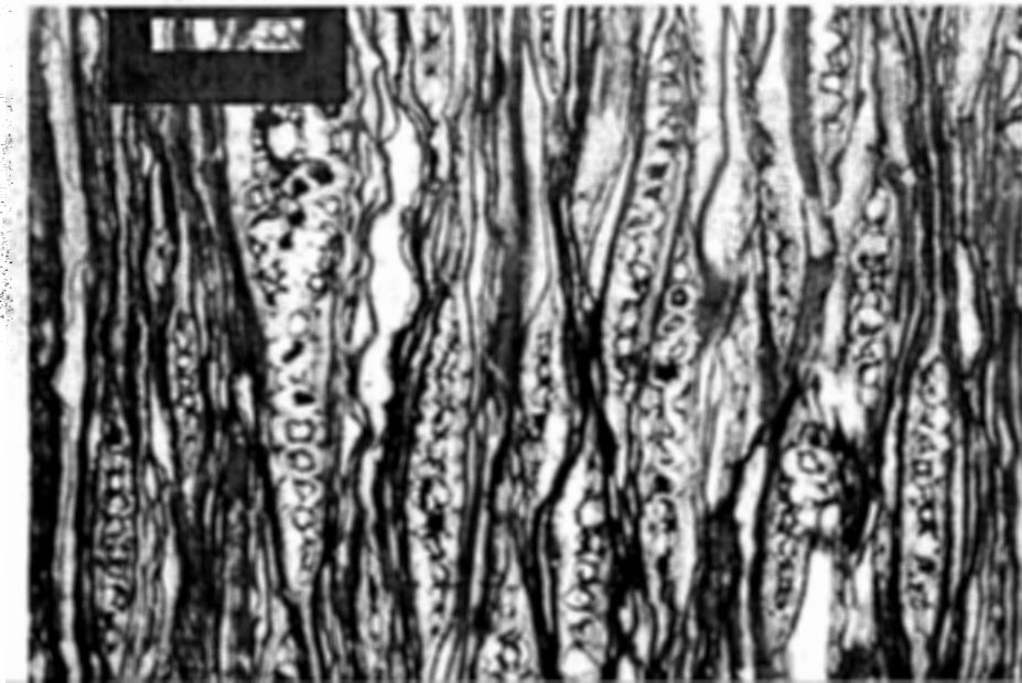
Figure 3.4: shows the various types of rays present in a sample. (EL87-257) Scale bar represents 100 \mu\text{m} .
