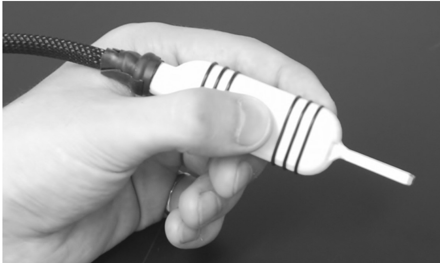
Figure 3-5: Photograph of the fully packaged endoscope with the 64 micro-coaxial cables exiting the proximal end of the flex circuits and passed through the rapid-prototyped plastic housing
