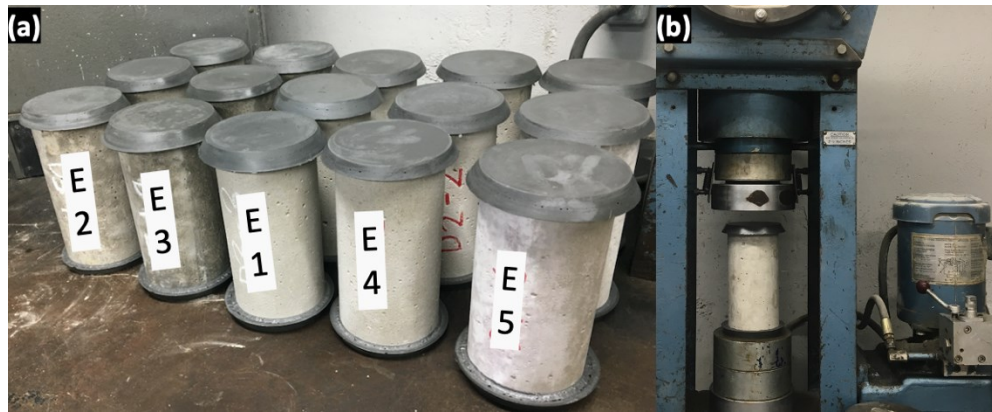
Figure 5-9 (a) A group of specimens after environmental conditioning to be tested under compression; (b) specimen prepared for compression test
