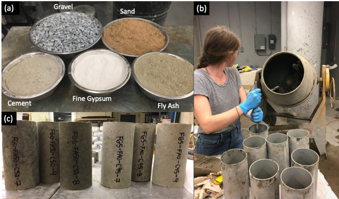
Figure 4-3 Specimen preparation: (a) dry materials; (b) hand tamping; (c) comparison of specimens with and without fly ash
