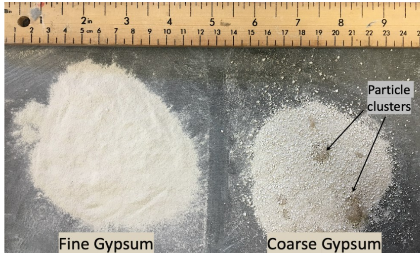
Figure 5-1 Comparison of fine and coarse gypsum material
