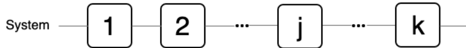
Figure 2.2: The object can also be interpreted as a series system with k independent but not identical components. T_j can be interpreted as the lifetime of the j^{th} component.
