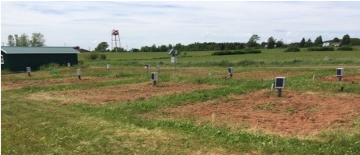
Figure 1. Lysimeter cells at Dalhousie Faculty of Agriculture Bio-Environmental Engineering Center.
