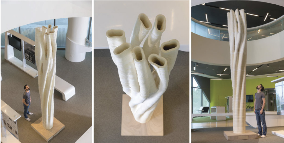
The FLAM project, 3D printed panel system in cellulose and chitin in large scale manufacture (Fernandez 2018)
