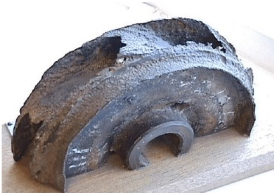
Figure 1.21 – Worn out impeller of centrifugal pump
