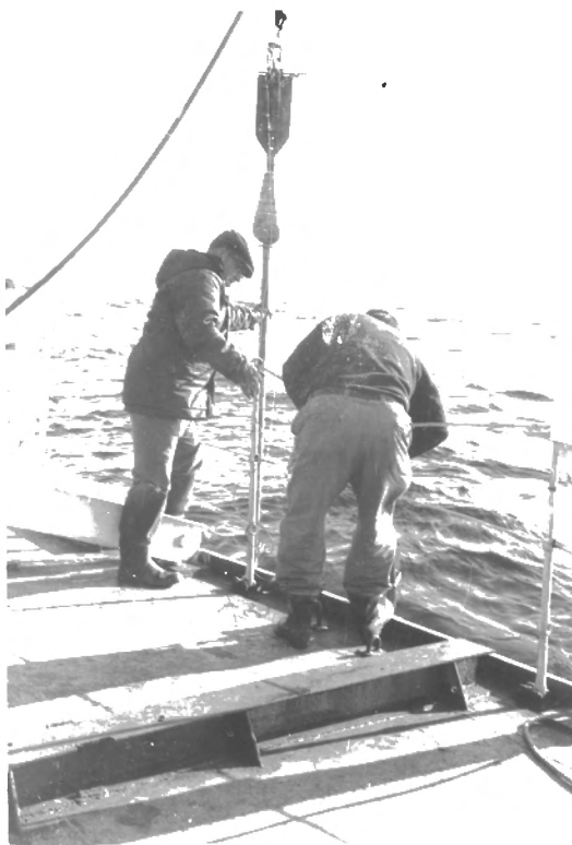
a. Laying out trigger weight.
