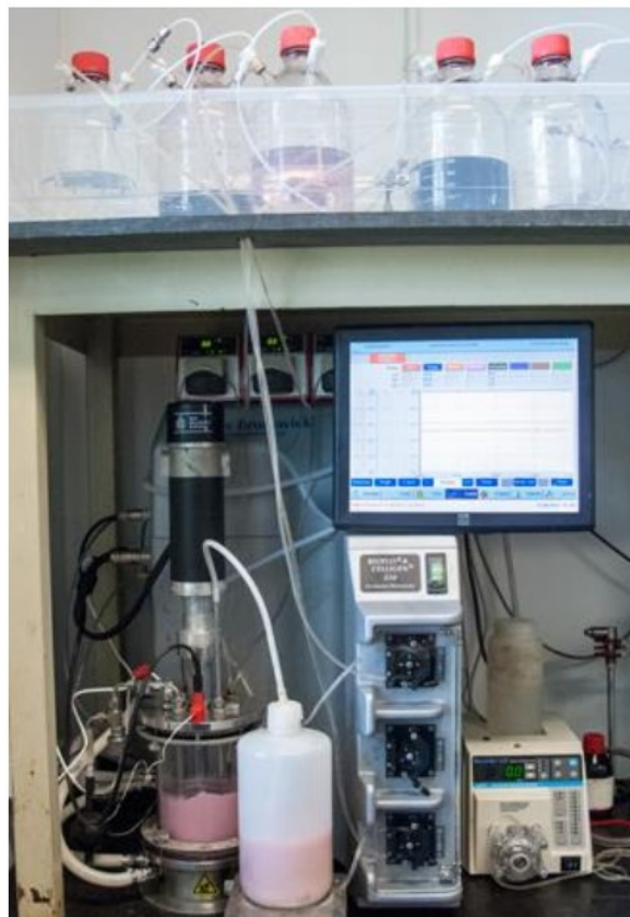
Figure 3.1 Schematic of a typical CSTR co-precipitation system
