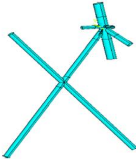
Figure 5-13: Model of the cross diagonal brace substructure [42]
