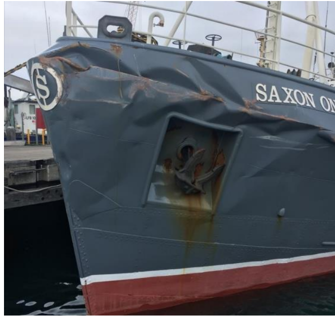
Figure 4-4: Deformation of Saxon Onward resulting from bow collision [29]
