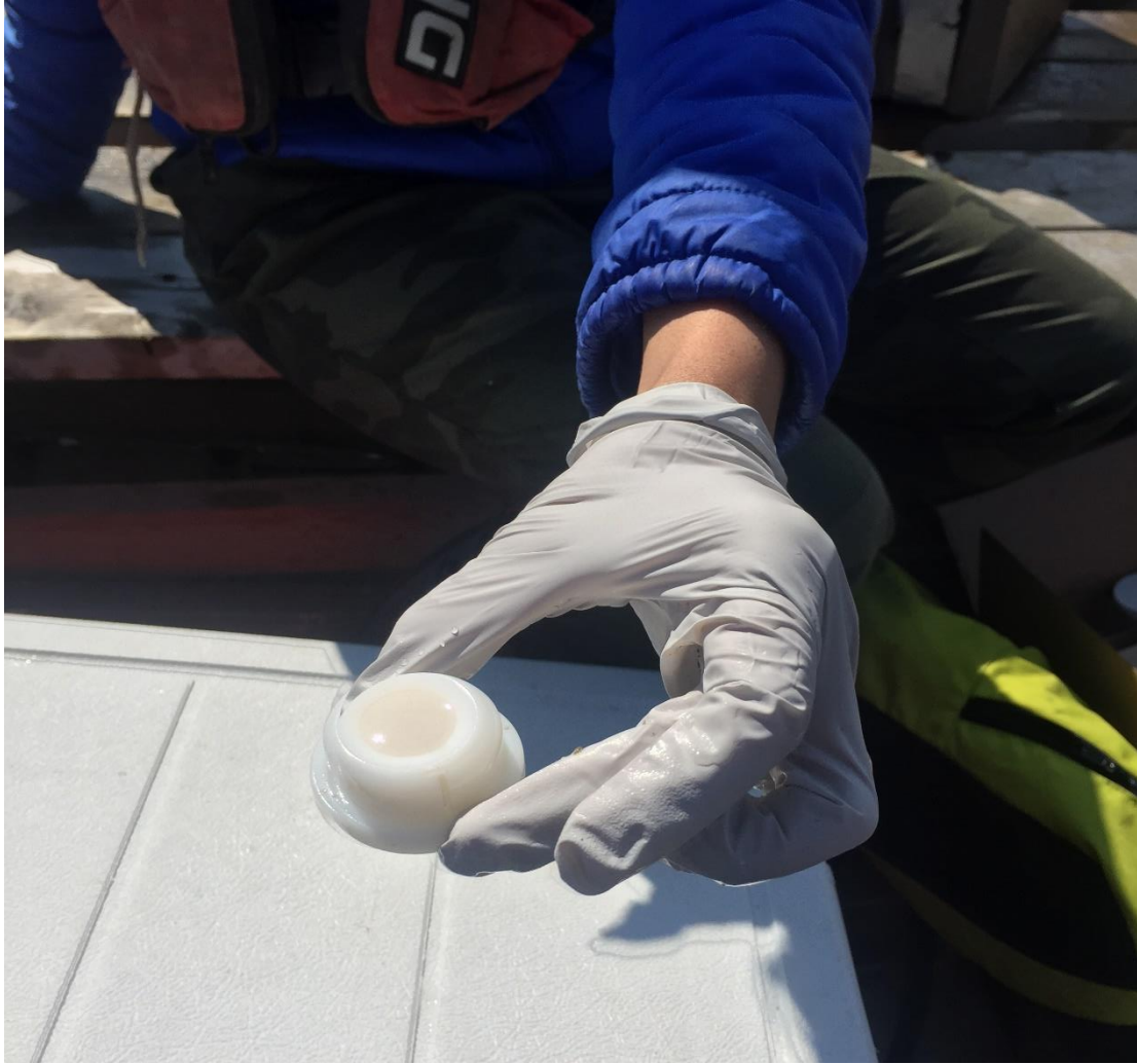
Image 10. Diffusive gradient in thin films sediment probe disc.
