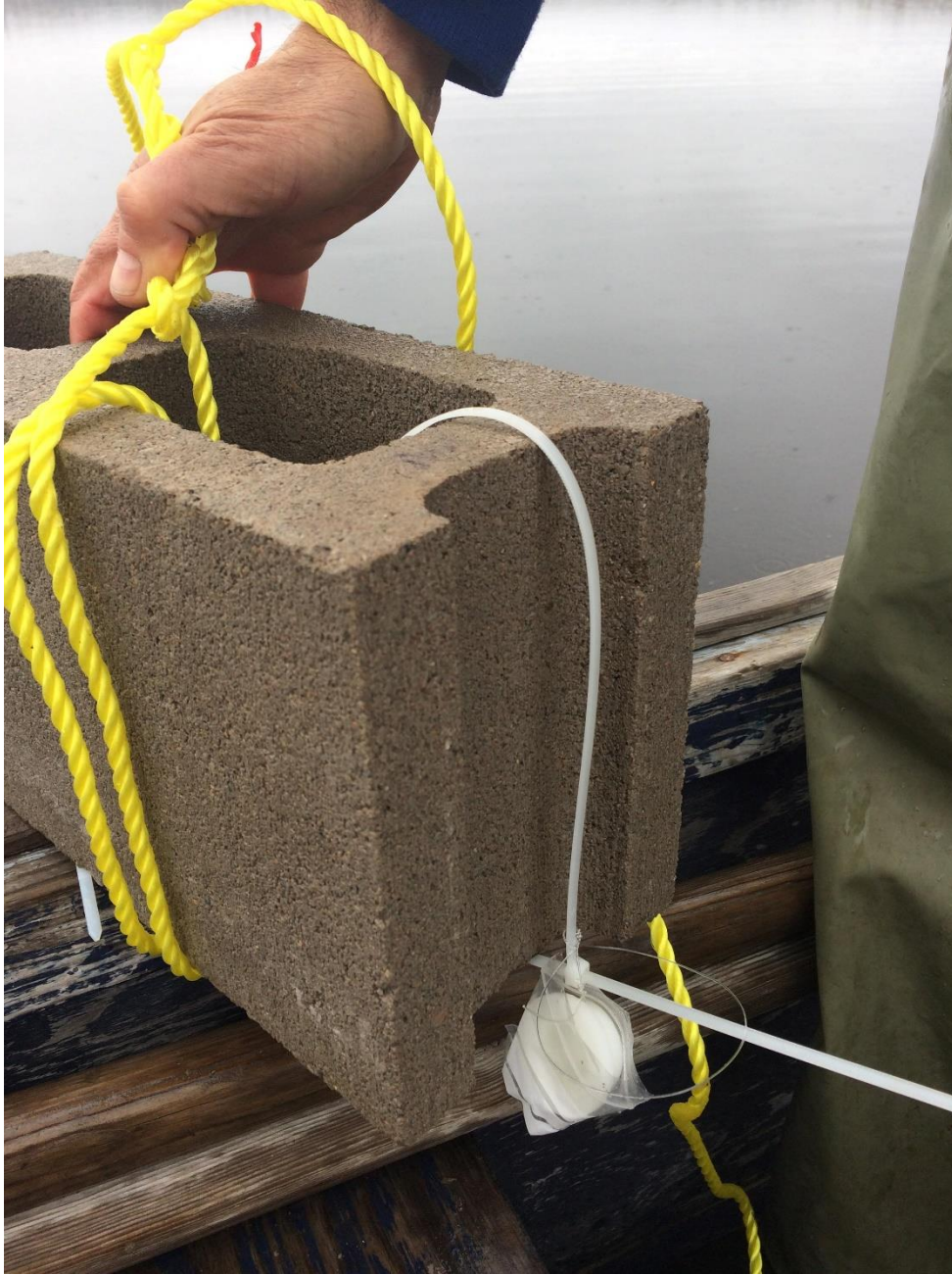
Image. 11 DGT disc tied to cinder block and plastic cable ties.
