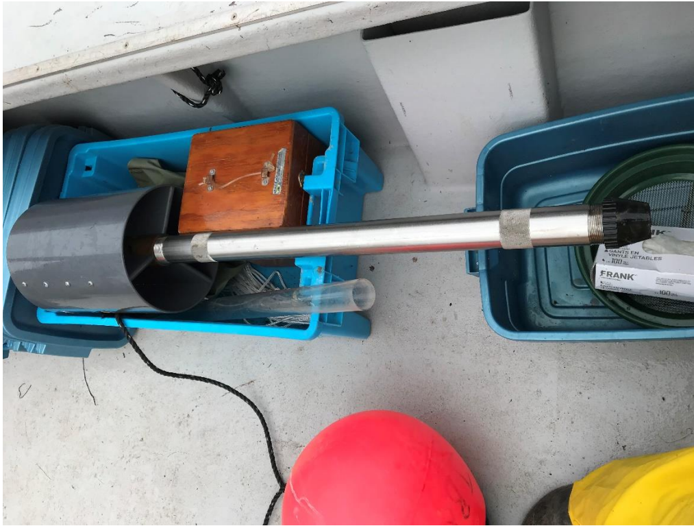
Image.2. Long gravity corer 2416 B45 (Wildco®) used for sediment sampling.
