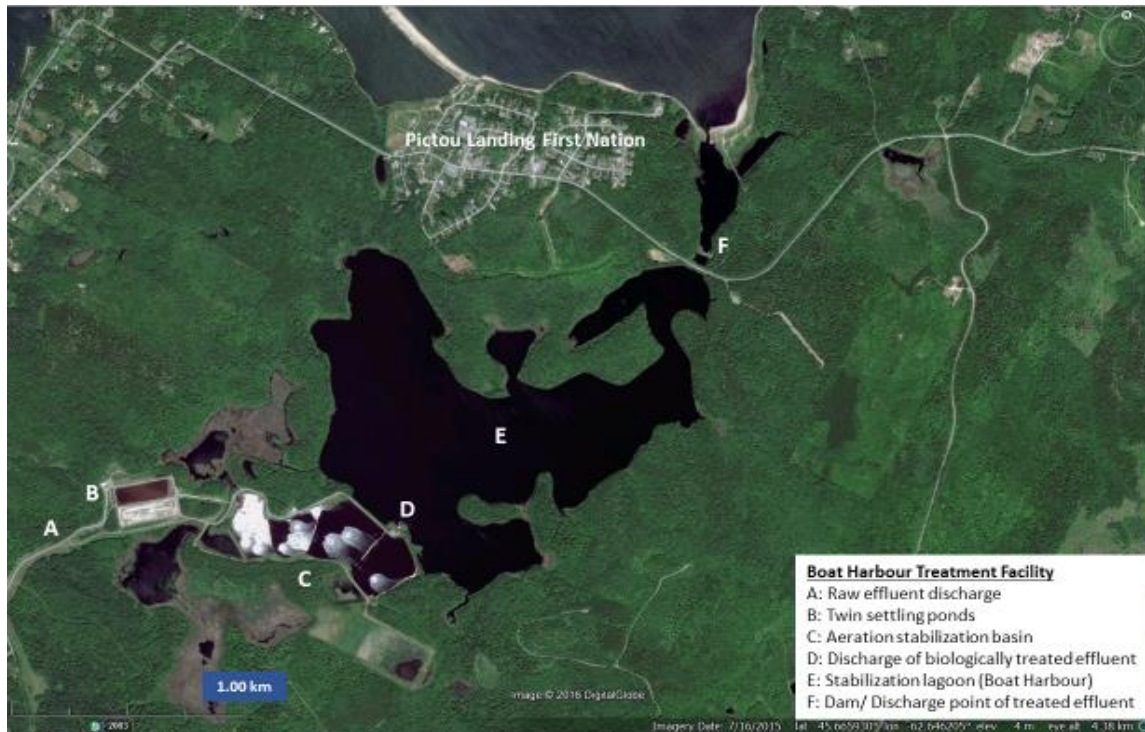
Fig. 2. Components of Boat Harbour Treatment Facility (BHTF) (from Hoffman et al. (2017a)).
