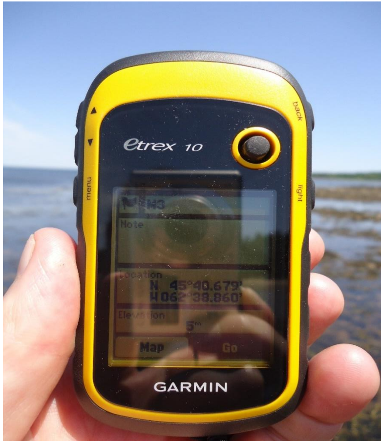
Image.1. Garmin GPS unit for recording waypoints of sampling stations.
