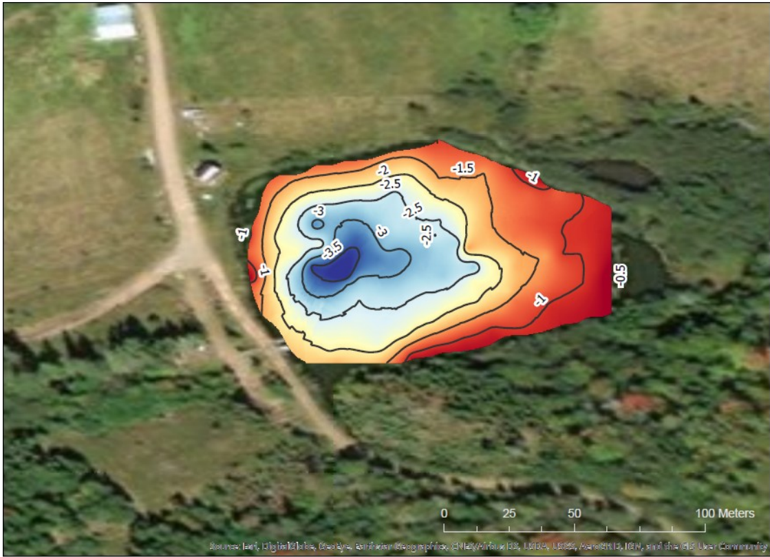
Figure A1. Bathymetric map of the Upper pond at North River Fish Farms Ltd. Measurements (m) were taken on June 18, 2018.
