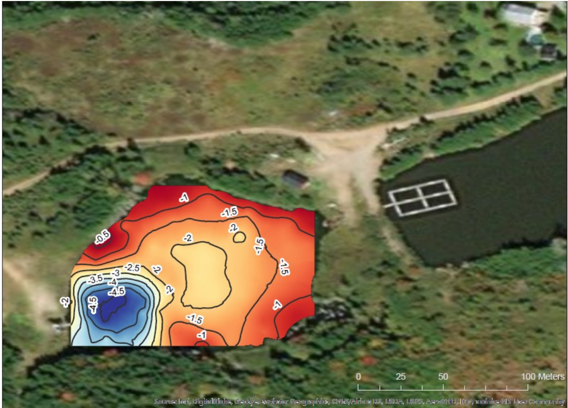
Figure A3. Bathymetric map of the Lower pond at North River Fish Farms Ltd. Measurements (m) were taken on August 29, 2017.
