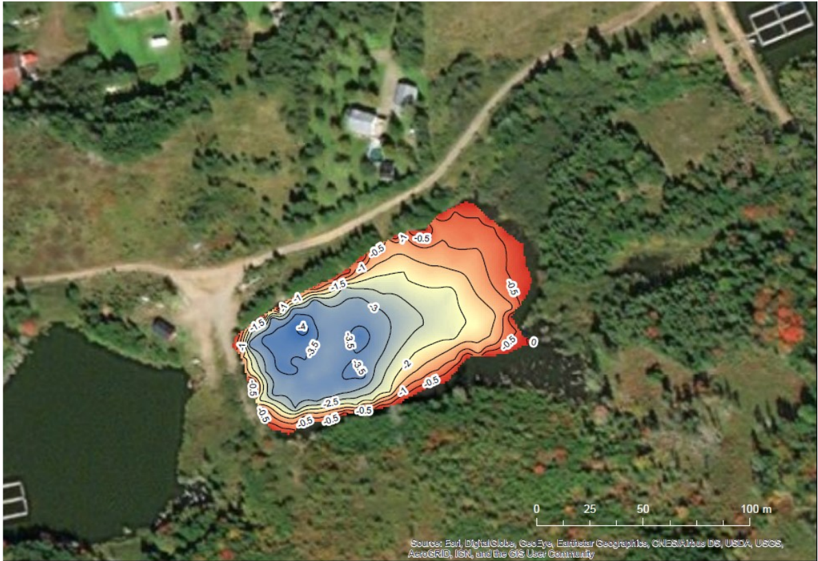
Figure A2. Bathymetric map of the Middle pond at North River Fish Farms Ltd. Measurements (m) were taken on August 29, 2017.
