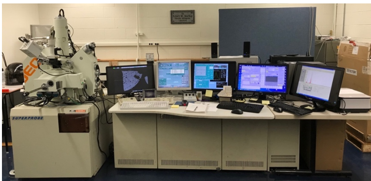
Figure 10 - Photo of JEOL EPMA 'SuperProbe' in Dalhousie University's Robert M. MacKay Microprobe Laboratory
