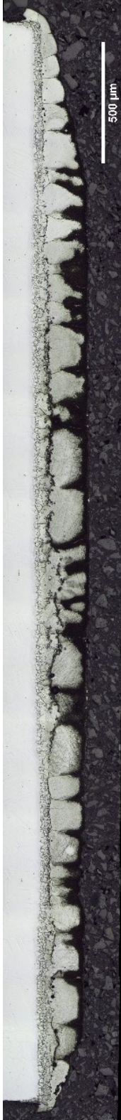
Figure 5.18 – Stitched composite micrograph of Ni30/IN625 wide gap half braze joint held at 1050 °C for 240 minutes. Examined braze joint width is 4.5 mm. Darkly etched region is the S region.
