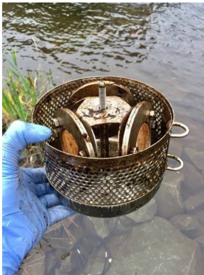
Figure 14. POCIS taken from Lake Fletcher after the 28-day exposure time.
