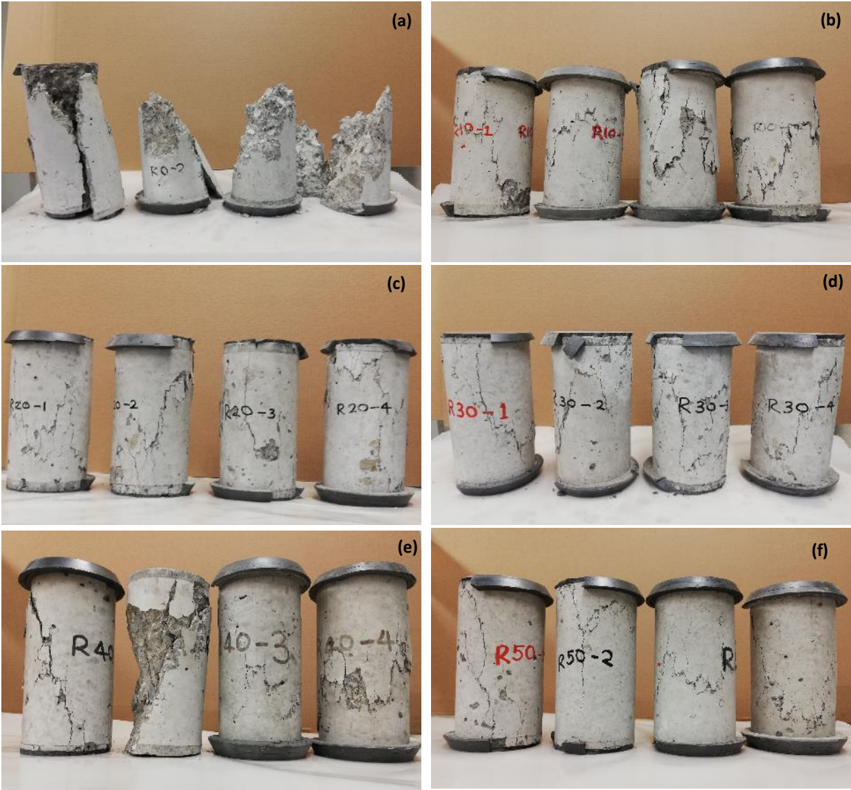
Figure 5: Failure mode of specimens: (a) R0; (b) R10; (c) R20; (d) R30; (e) R40; and (f) R50
