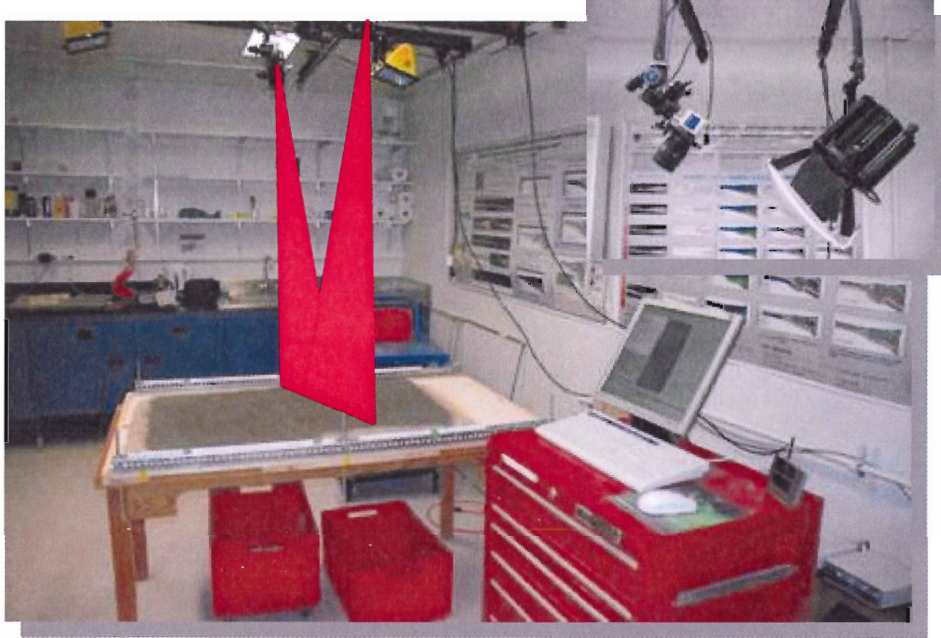
Figure 1.4 General view of PIV setup of analogue experiment. Cameras and lights setup above experiment for monitoring of surficial deformation. Red triangles indicate the viewing direction of the stereoscopic cameras.
