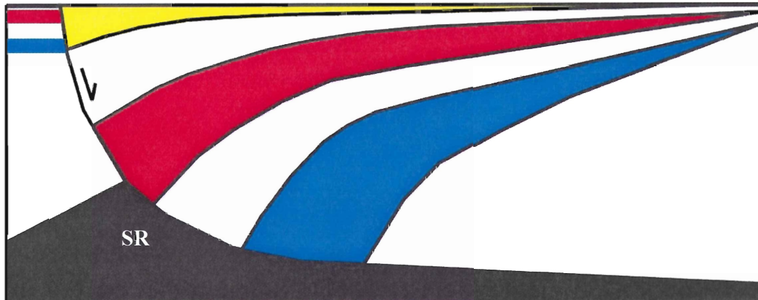
Figure 2.2 Diagram showing triangle shaped salt rollers (SR) occurring as extension and growth faulting takes place. Salt represented by black layer.
