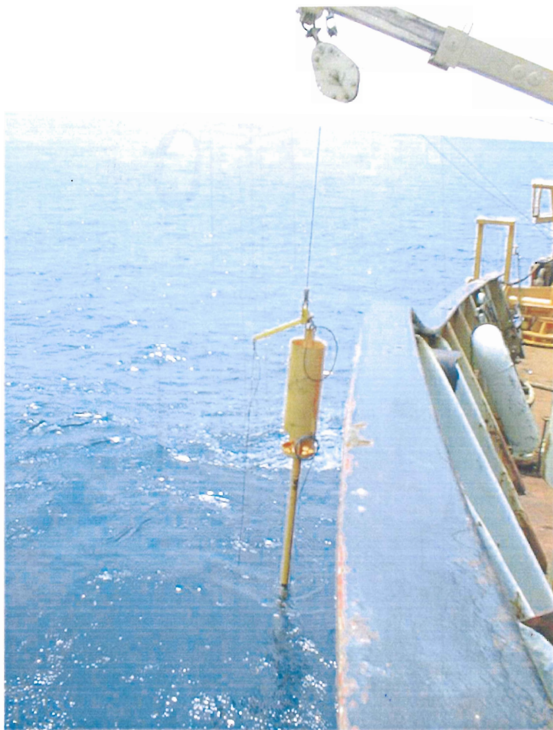
Figure 2.4 Piston Core deployment. (Photo from Hudson Cruise 2004)
