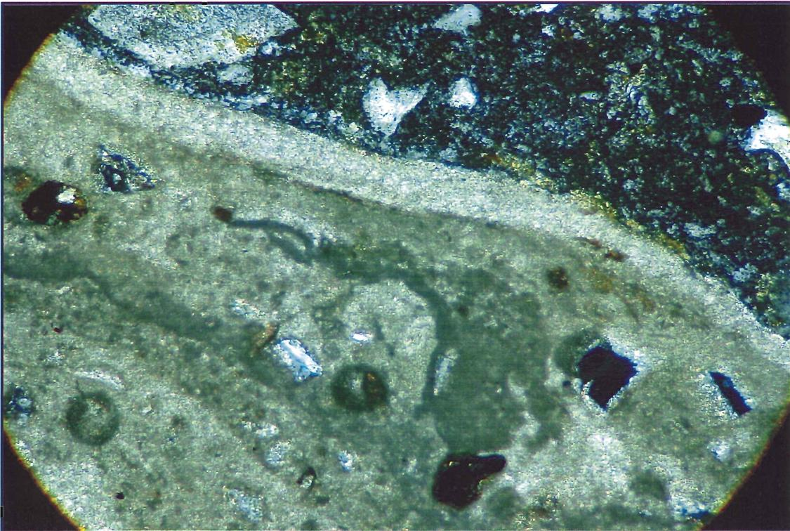
**Figure A1.4** The boundary between a large amalgamated central material zone, containing plagioclase and quartz as a fine grained matrix and interstitial grains.
