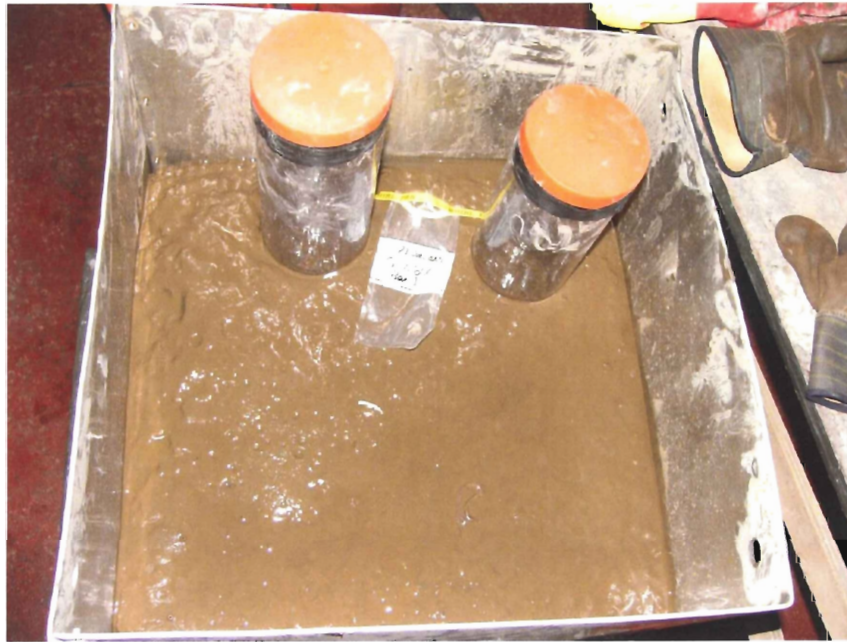
Figure 2.5 – Box core with push cores and surficial samples (CASES, 2004)
