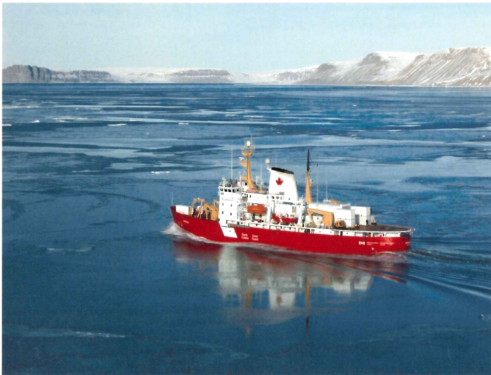
Figure 2.1 – CCGS Amundsen is a class 3 icebreaker refitted for arctic research (CASES, 2004)
