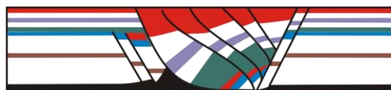
Figure 2-7: Triangle shaped salt roller/reactive diapir (black) and associated faults. (After Krezsek et al., 2006a)
