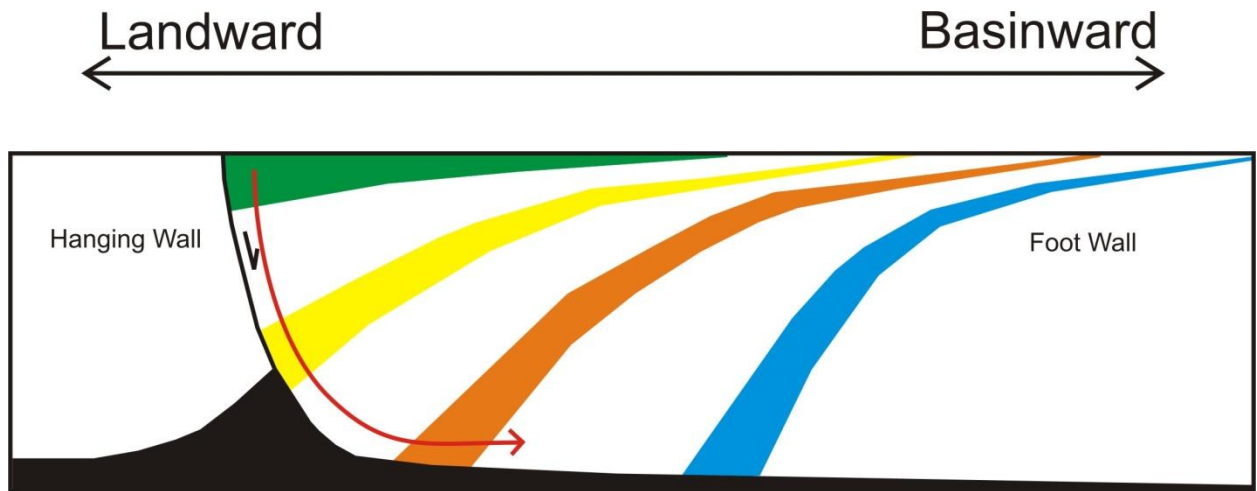
Figure 2-1: Basinward dipping growth normal fault. Thick packages of strata indicate growth of overburden from fault controlled subsidence. Salt is indicated by the color black and the sense of rotation is noted by the red arrow.
