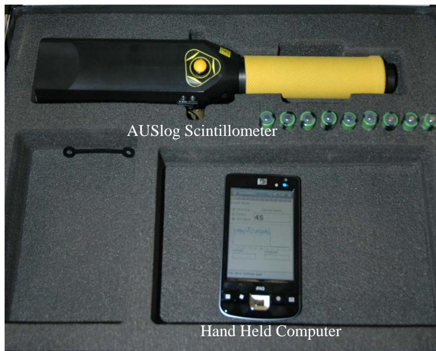
Figure 2.2: Photo of the AUSlog scintillometer.
