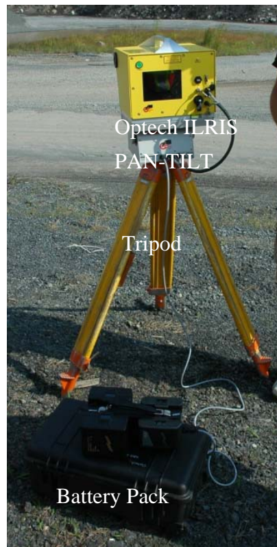
Figure 2.1: Photo of the Optech ILRIS LiDAR.
