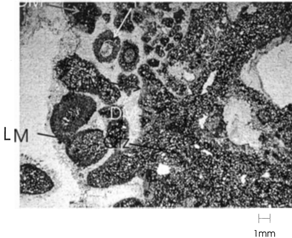
Figure 4.13: Two types of micrite are identified: (1) dark brown micrite-grade material (DM) and (2) light brown micrite (LM). The dark brown micrite-grade material is quartz rich (Qtz). Lime mud clasts have both types of micrite. Clasts with a large component of light brown micrite have a peloidal-like texture (P).
