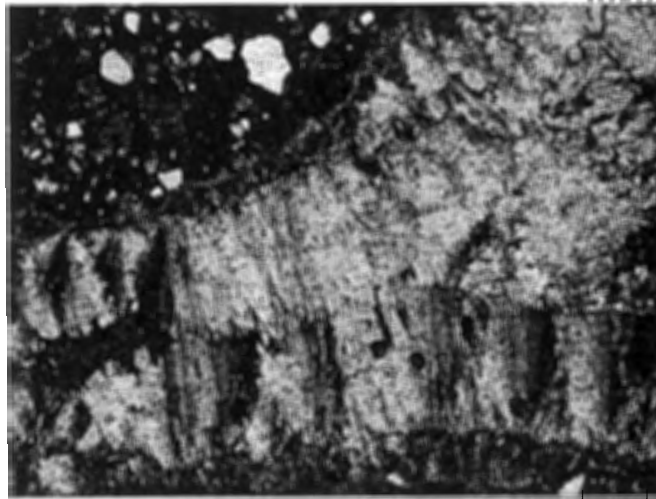
Figure 4.14: Three thin-sections of sparite. (A) Sparite occurring in a pore space. The sparite has a radial to bladed crystal form. (B) Sparite occurring in a pore space. The sparite has a radial crystal form. (C) Sparite occurring on the surface. The sparite has an acicular crystal form. The sparite is concentrically banded.
