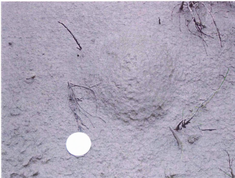
Figure 4.3b Picture of the bubbles forming in the cyanidation tailings on the edge of the ponds (Picture taken by M. Parsons, 2003).
