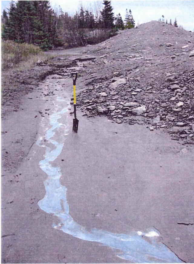
Figure 4.3a Picture of the rivulet on the cyanidation tailings that contains the white precipitate (Picture taken by M. Parsons, 2003).
