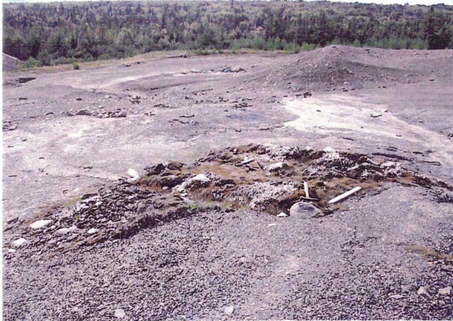
Figure 4.2a This overview picture of the younger tailings shows the moss growing on the surface where the cyanide drums and lime were buried with the blue efflorescent salt in the distance (Picture taken by M. Parsons, 2003).
