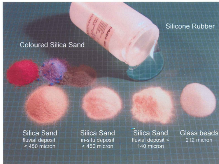
Figure 2.2: Materials used in analogue models at Dalhousie University. This thesis uses only the silicone rubber, fluvial silica sand, and coloured fluvial silica sand.
