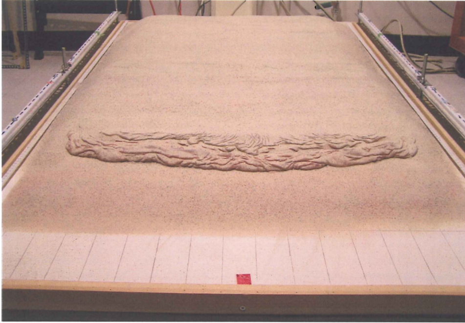
Figure 1.12: Frontal salt tongue canopy, as seen from the surface of the model, near the end of the experiment, from experiment 4-2.
