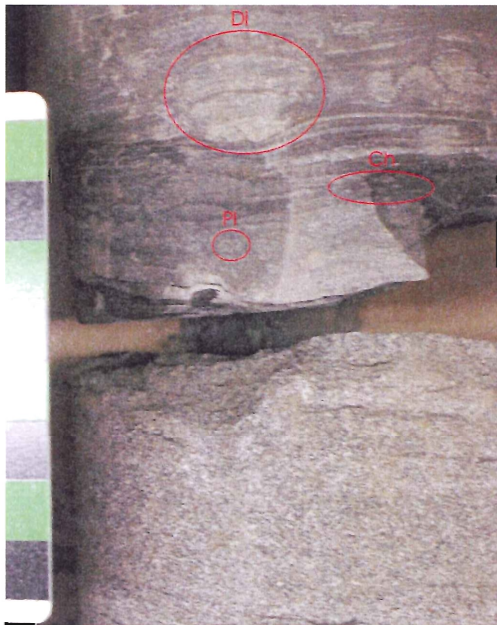
Figure 4.5.2. Upper contact between the Bluesky Formation and the overlying Wilrich Member. The upper shale portion has a high sand content and appears as a gradational contact. The shale contains trace fossils Thalassinoides , Planolites , and Chondrites . The sandstone portion of the photo has a salt and pepper appearance possibly due to a higher chert content. (Photo by Scott Doyle, 2005).
