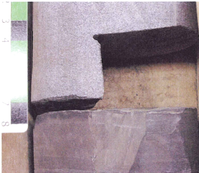
Figure 4.6.6. The lower sand/shale contact within the Bluesky Formation. This shale separates the Bluesky Formation from the Gething Formation. The sand in this photo has much less glauconite and has a salt and pepper appearance. (Photo by Scott Doyle, 2005).
