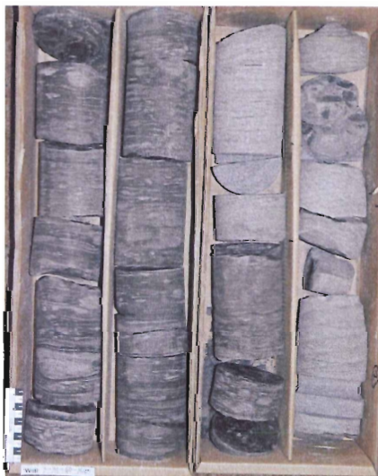
Figure 4.4.2. The top two boxes ~ 3.00m of core from this well. The core shows both reservoir quality sands as well as high mud content sands. The core top is located in the top right corner of the photo and the bottom of this section in the bottom left of the photo. All of the tops are in the top of the photo and move in sequential order from right to left. In the core there are visible crossbedding, organic materials, and trace fossils. (Photo by Terrance Lukie, 2005).
