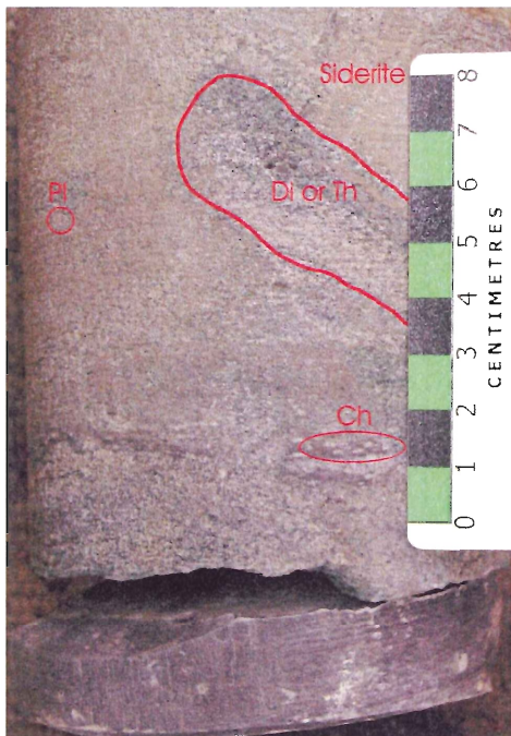
Figure 4.5.6. The lower sand/shale contact within the Bluesky Formation. The contact is sharp and may represent incision of the Bluesky into the underlying shale. The sands contain trace fossils Thalassinoides or Diplocraterion , Chondrites and Planolites , as well as siderite cement and abundant glauconite. (Photo by Scott Doyle, 2005).
