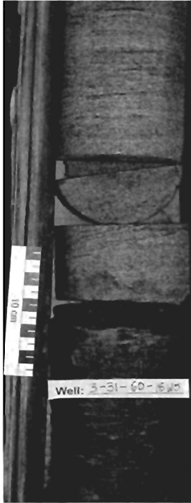
Figure 4.4.3. Shale/sand contact at ~2051.5 m. The contact is very sharp with a cross bedded sandstone on the right and a mudstone on the left. The shale appears somewhat more fissile at the contact. This sharp contact may indicate a regressive event. (Photo by Terrance Lukie, 2005).
