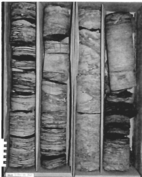
Figure 4.4.4. The middle two boxes ~3.00 m of core from this well. The top of the core is in the top R corner of the photo and the bottom of the core in the bottom L corner. All tops are in the top of the photo and are sequential from right to left. The core has high mud content, is very highly bioturbated, and contains many mud laminae and drapes. There is a section of fissile shale more than half way down the first section of the core. The next section shows some traces and possibly some sediment loading features. (Photo by Terrance Lukie, 2005).
