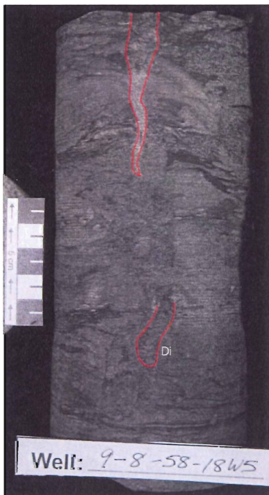
Figure 4.3.2. Mudstone with a high sand content. The U shaped burrow at the bottom of the core is a Diplocraterion trace fossil, while the long narrow burrow at the top may be Arenicolites or Skolithos . (Photo by TerranceLukie, 2005).
