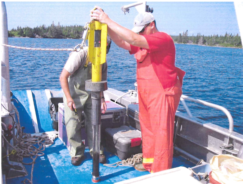
Figure 3.3 Gravity corer used for the collection of sediment cores in Wine Harbour (Photo taken by M. Parsons, 2004).
