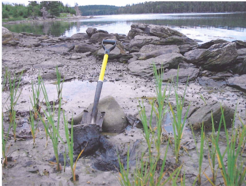
Figure 4.3b Tailings sample site T9, in the intertidal zone. The tailings here are unoxidized, giving them a characteristic dark grey colour (Photo taken by M. Parsons, 2005).
