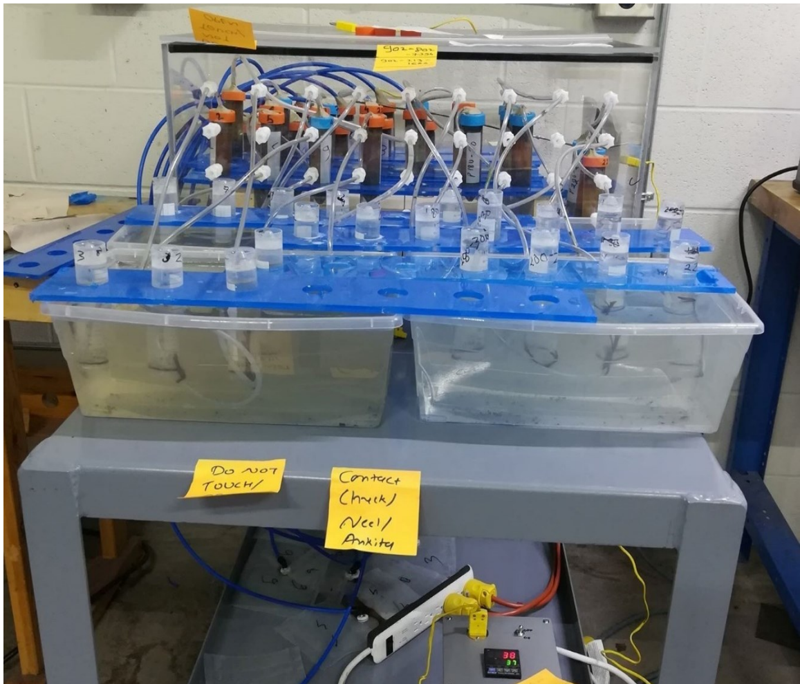
Figure 4.13 Experimental Setup for Anaerobic Co-digestion of the processed water
