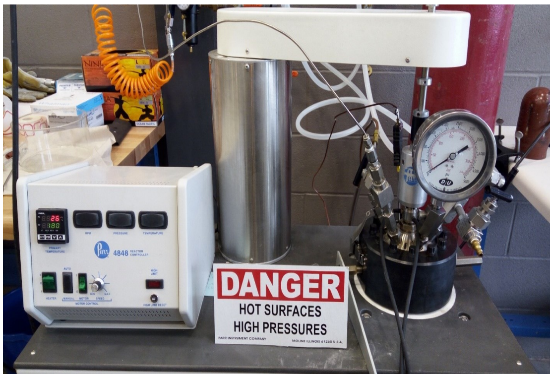
(a) Batch reactor system with the controller (PARR 4571 High-Pressure High-Temperature Reactor System with PARR 4848 Reactor Controller)
