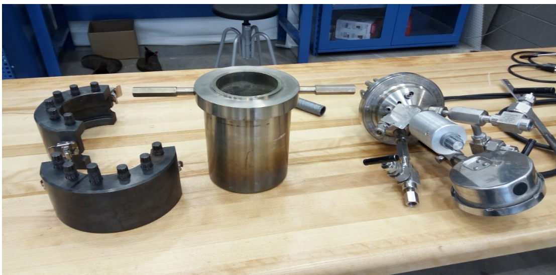
(b) The reactor container and the movable head
