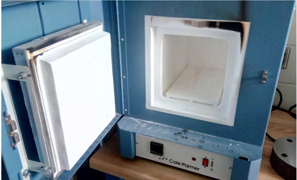
Figure 3.6 Muffle Furnace which was used to carry out the proximate analysis of the hydro-char samples (Cole-Parmer StableTemp OF-33858-60)
