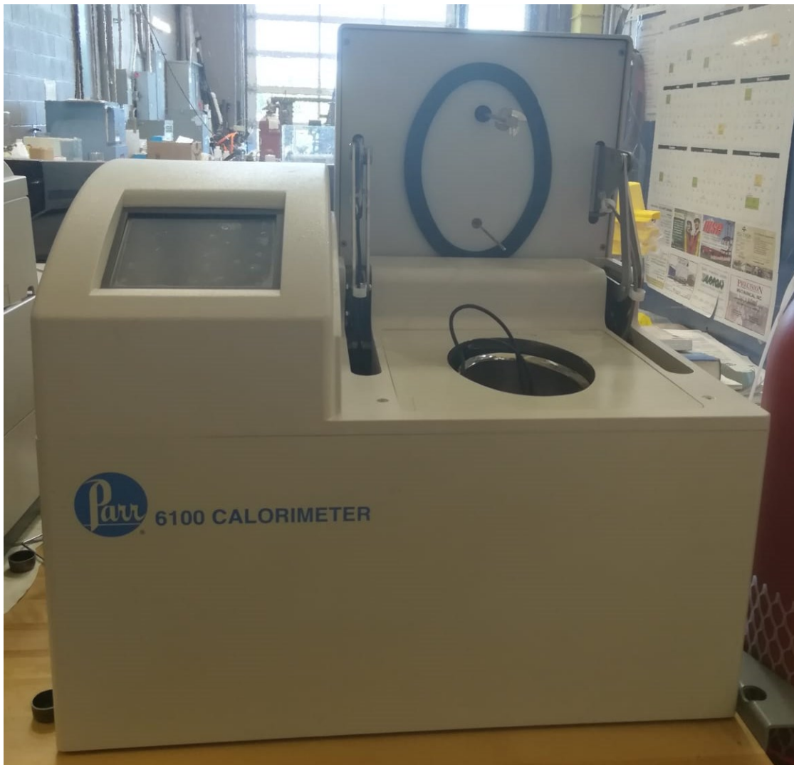
Figure 3.8 The Bomb Calorimeter that is used for calculating the HHV of the hydro-char samples (Parr 6100 calorimeter)
