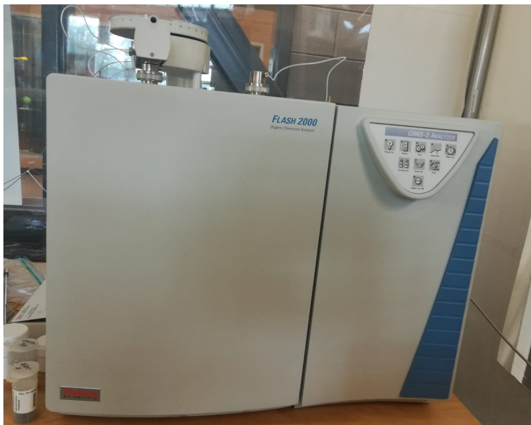
Figure 3.7 CHNS-O Analyzer that is used to perform the ultimate analysis of the hydro-char samples (Thermo Fisher Flash 2000 CHNS-O)
