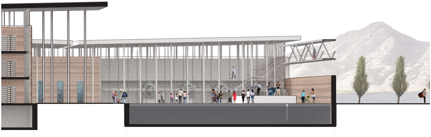
Detail of section through clear well and pedway with water treatment building behind.
