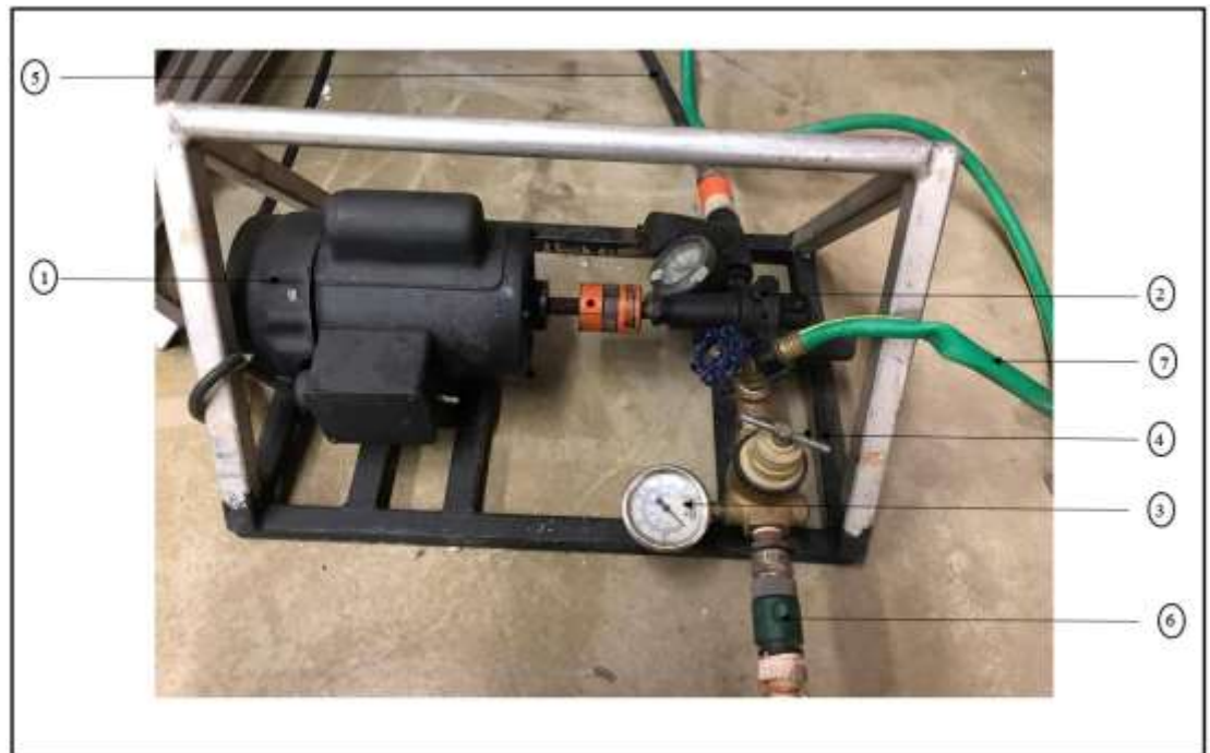
1. Electric motor 2. Pump 3. Pressure gauge 4. Flow control valve 5. Suction pipe 6. Delivery pipe 7. Bypass.
