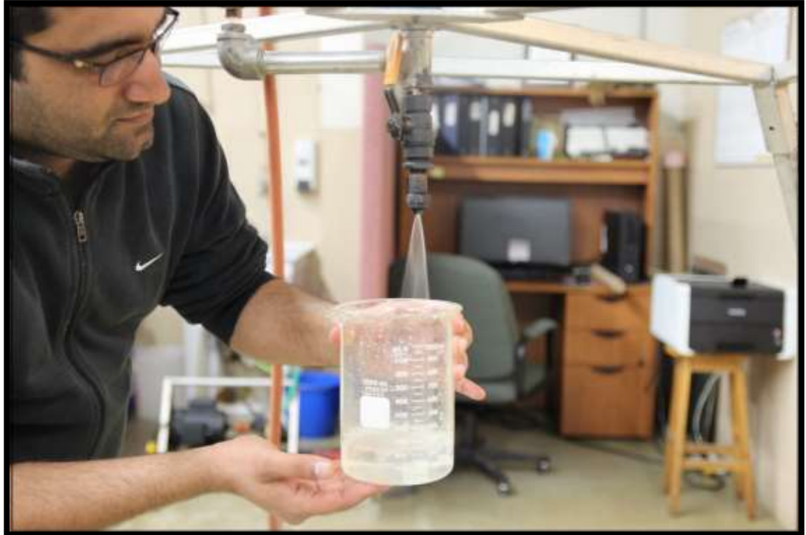
Figure 2-6: Collection of volume of water from nozzle at different pressures
