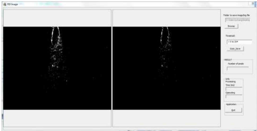
Figure 2-4: Image processing program that segments a PIV image to black/white image using different threshold values (0 to 254)
